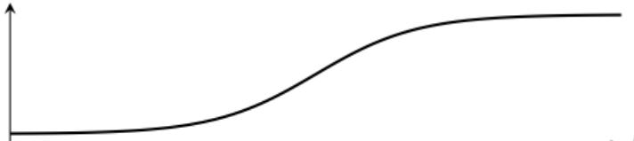
*Purpose:* Map to (0, 1) for probabilities (binary outputs). Can saturate/vanish.
